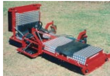
The TM372, wing deck mower, fitted with a large diameter, short front roller and rear, solid rubber wheels.
